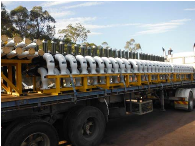
Upstream Water & Gas Riser Legs - QCLNG
