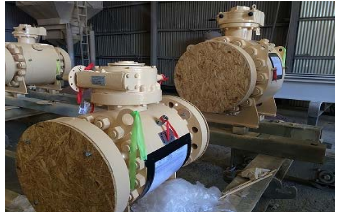
400nb 1500# Painted Valves during Final Inspection
