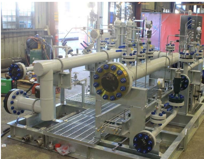
Oil / Gas Wellhead Metering Skid - Oil Search
