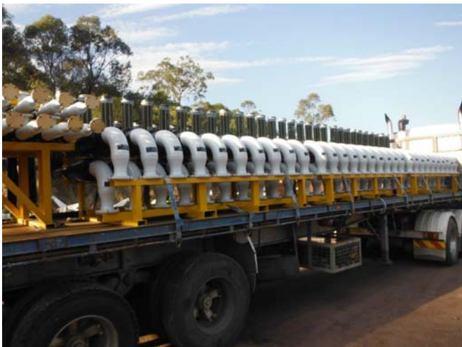
Upstream Water & Gas Riser Legs - QCLNG
