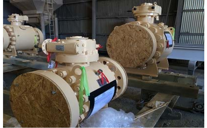
400nb 1500# Painted Valves during Final Inspection
