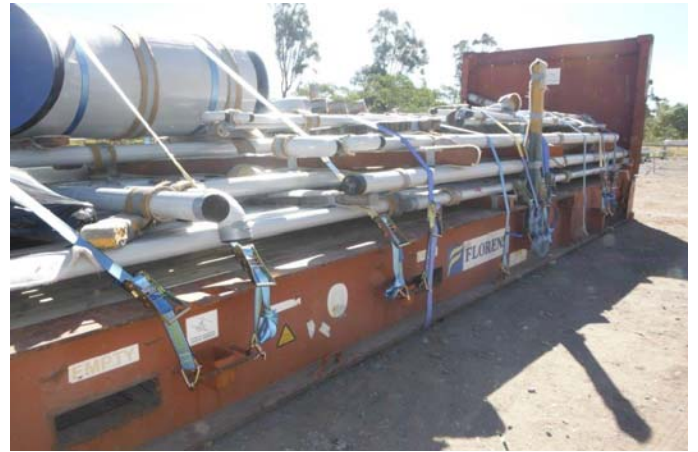
Gas Piping packaged on Flat Racks - APLNG
